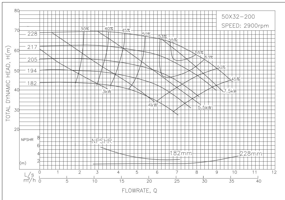
Performances for standard construction, clean cold water. Performance correction for Stainless Steel construction 4%.
