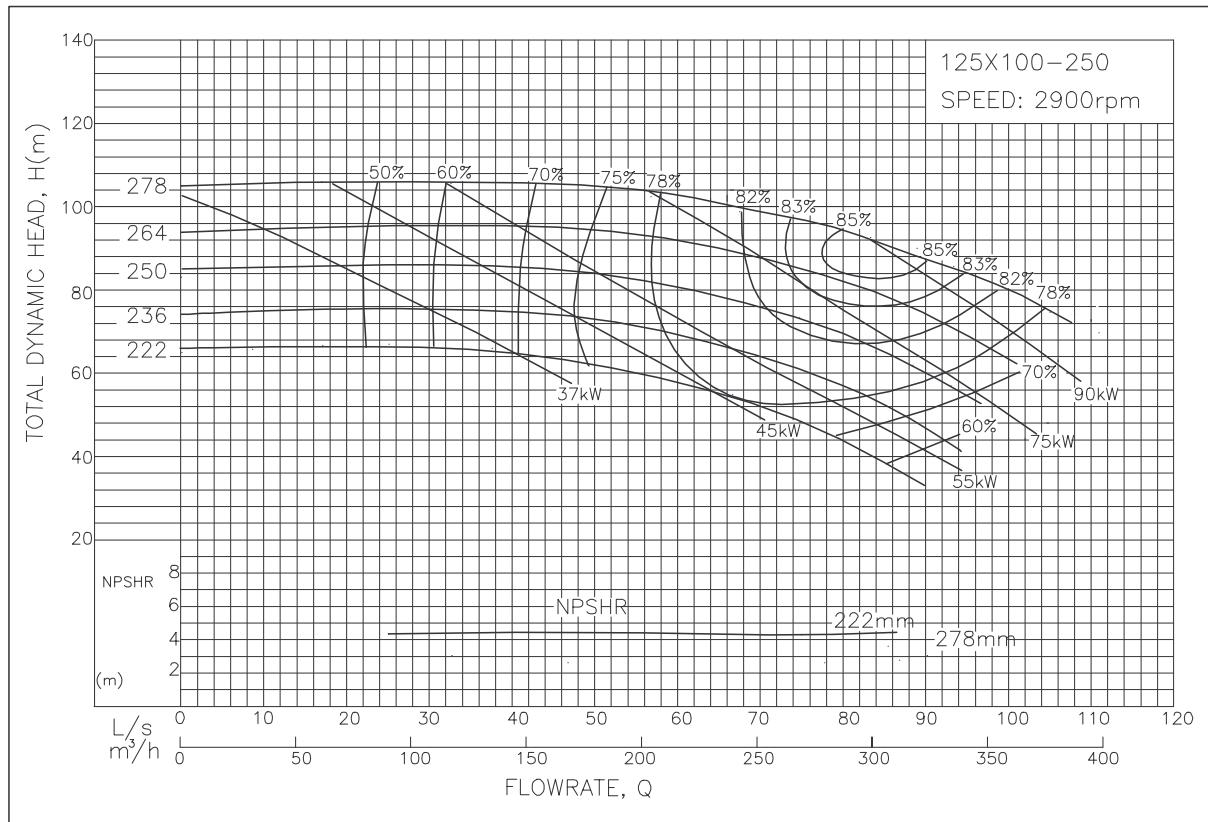
Performances for standard construction, clean cold water, efficiency correction for Stainless Steel construction 4%.
