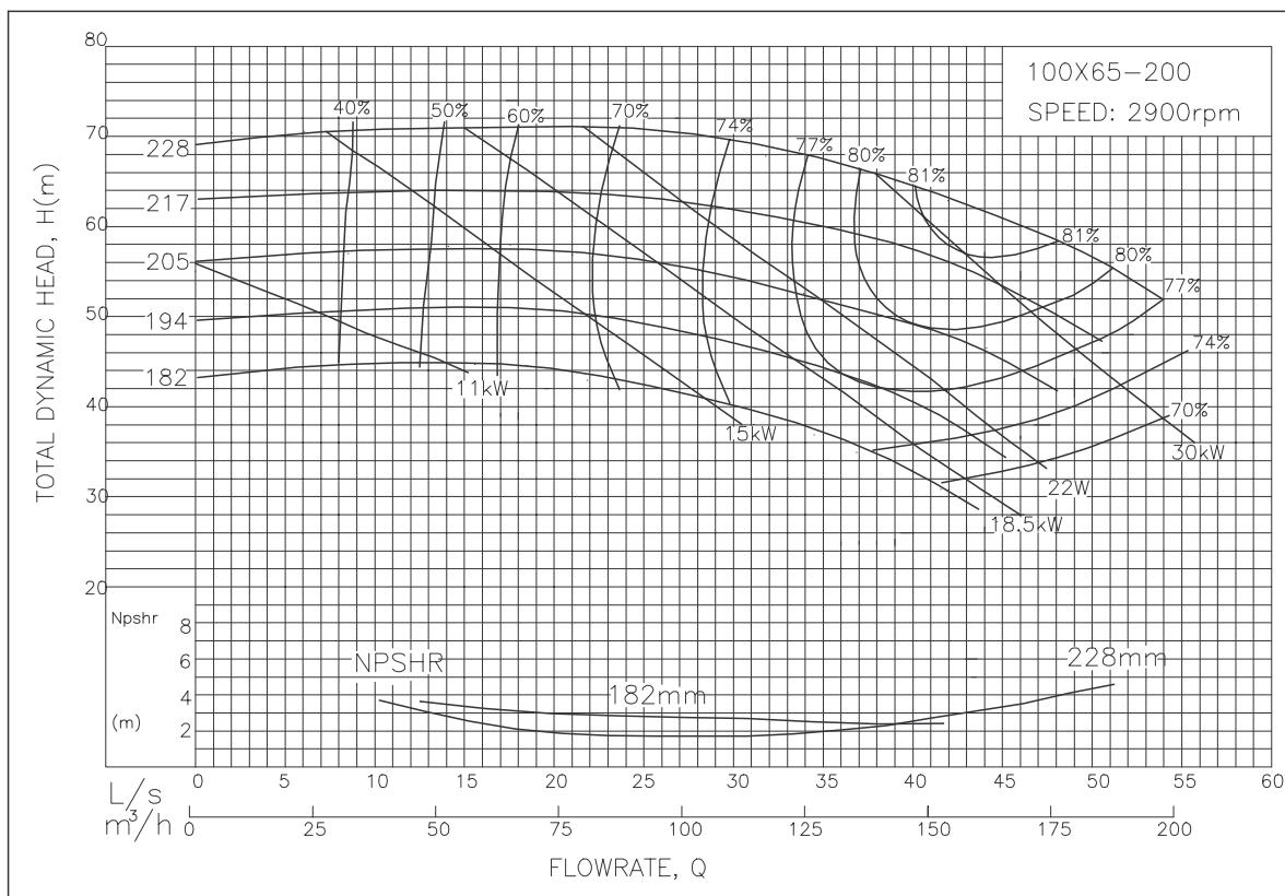
Performances for standard construction, clean cold water, efficiency correction for Stainless Steel construction 4%.
