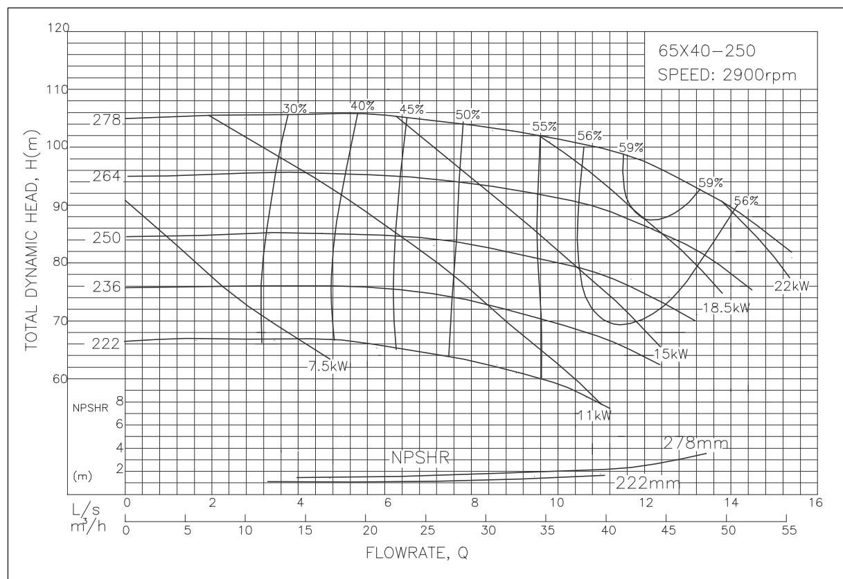
Performances for standard construction, clean cold water. Performance correction for Stainless Steel construction 4%.
